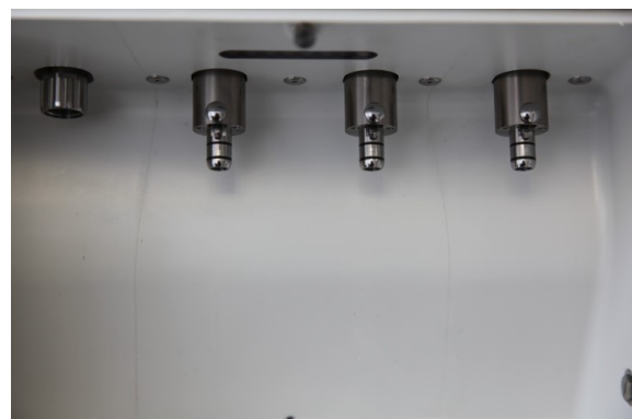
Fig.18 – iCare+ C3: coupling for 3 contra-angles
